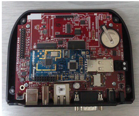
Fig. 3. Gateway. Single board with a mote attached.
